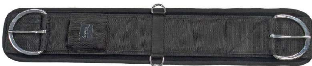
8502 - Western Girth, washable Neoprene. The web is velcro stuck to the neoprene and hence the system can be separated for washing, 3" stainless steel buckles. Sizes: 70cm to 100cm
